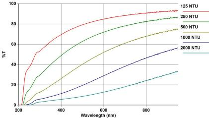
Diffuse transmission of formazin standards (125 to 2000 NTU (= Nephelometric Turbidity Unit)) measured using the Agilent Cary 60 UV-Vis DRA to assess light scattering behavior. Each measurement was performed using the standard 10 mm cuvette holder. Formazin is widely used to assess turbidity in water quality testing and to evaluate clarity of juices, beers, and dairy products, where haze formation can impact product quality.
