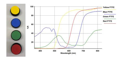
Diffuse reflection of colored PTFE diffuse color standards measured using the Agilent Cary 60 UV-Vis DRA. The standards support manufacturers in achieving consistent color reproduction of products such as textiles, papers, pharmaceuticals, paints, and inks.
