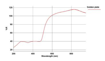
Specular reflection of a gold-coated mirror measured using the Agilent Cary 60 UV-Vis DRA with the 8° port reduced holder.
