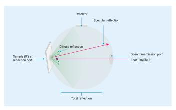
Schematic showing how reflectance measurements are performed using the Agilent Cary 60 UV-Vis DRA. The sample is mounted at the reflection port of the DRA, ensuring efficient collection of the diffusely reflected light (green). Although commonly referred to as a "diffuse reflectance accessory", the DRA allows users to exclude or include the specular component of reflected light, providing the flexibility to choose between diffuse-only or total reflectance measurement modes.
