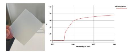
Diffuse transmission measurement of a frosted plastic packaging film designed to block UV light. The Agilent Cary 60 UV-Vis DRA ensures optimal light collection, capturing all scattered light for comprehensive characterization of the material.
