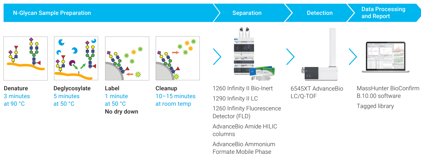
Figure 1. Released N-glycan analysis workflow using Gly-X InstantPC sample preparation with LC/FLD/MS.
