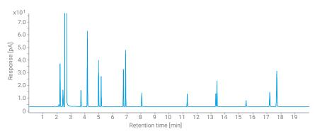
The 8850 GC equipped with a DB-1701 column and using helium as the carrier gas, exhibits outstanding performance in analyzing the 13 key components in the electrolyte.
