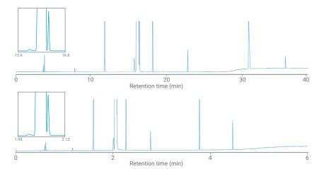
The 8850 GC offers the flexibility to run conventional methods using helium carrier gas (top) or fast methods using hydrogen carrier gas (bottom). Insets show D7504 p-xylene and m-xylene resolution requirements are easily met using either approach.
