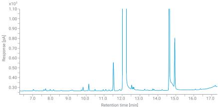
The 8850 GC, coupled with OpenLab CDS, accurately quantifies NMP solvent purity and monitors trace-level known and unknown impurities.
