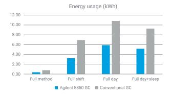
The 8850 GC used 45% less energy than conventional GC systems in this analysis of pesticides.
