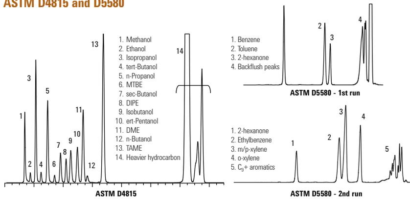
Here, dual parallel channels were configured on one GC system. Both oxygenates and aromatics were precisely determined in gasoline.
