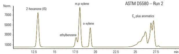
Overlay of 5 samples prepared with the Agilent 7696A Sample Prep WorkBench. This method measures benzene (0.1-5%), toluene (1-15%), C<sub>8</sub> aromatics (0.5-10%), C<sub>9</sub> plus aromatics (5-30%), and total aromatics (10-80%)
