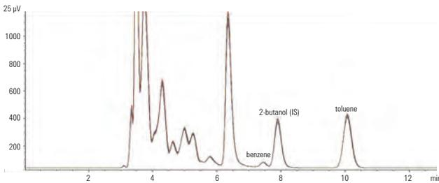
This overlay represents 10 samples prepared with the Agilent 7696A Sample Prep WorkBench. EPA method standards specify 0.1-5.0 vol% for benzene and 2-20 vol% for toluene.
