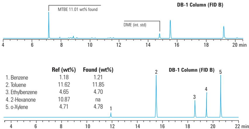
This analysis used Capillary Flow Technology (CFT) Deans Switch to simplify method setup, eliminate carryover, and minimize peak tailing for very polar compounds. Backflush was also used to reduce analysis time.
