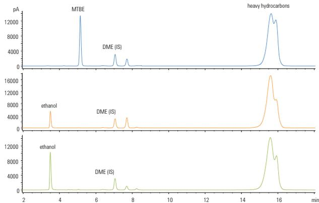
14 different ethers and alcohols from 0.1-15 wt% were detected. Samples were prepared with the Agilent 7696A Sample Prep WorkBench.
