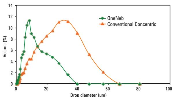
The OneNeb nebulizer (green) creates an aerosol with smaller droplets and a narrower size distribution than a conventional Conical nebulizer (orange). This ensures better precision and improved sensitivity.
