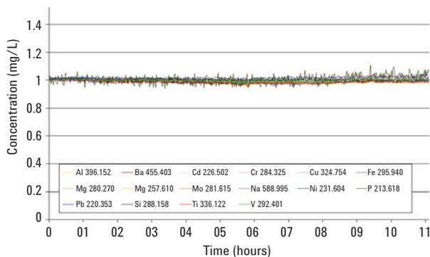
**Excellent chemical resistance:** Here you can see proof of the OneNeb nebulizer's long-term stability – even during continuous aspiration of ShellSol (low aromatic, inert hydrocarbon solvent).
