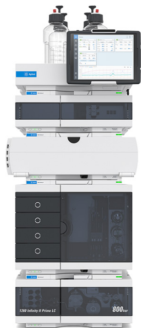
Figure 1. The two USP methods required for the analysis of pregabalin—assay and enantiomeric purity—are run on a single Agilent 1260 Infinity II Prime LC instrument, which contains technology from the Agilent 1290 Infinity II LC System. The methods use different columns, so a column selection valve was employed so that no manual method switchover of the LC was required.
