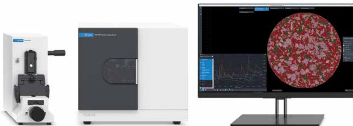
(from left to right) the Agilent Sample Planer, Agilent 8700 chemical imaging system, and Agilent Clarity software.
