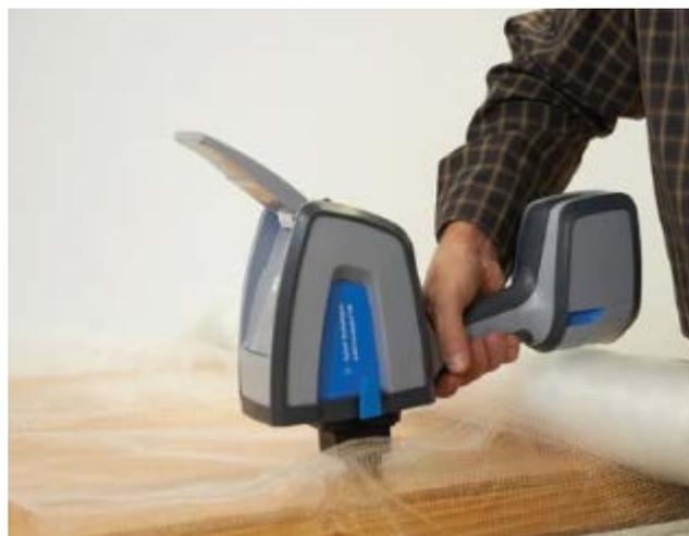
The 4300 Handheld FTIR is the first of its kind combining lightweight ergonomics, ease of use, ruggedness, and flexibility into one system. The 4300 weighs in at approximately 2 kg. With its light weight and ergonomic design it's ideal for field use and deployment into non-laboratory situations.
