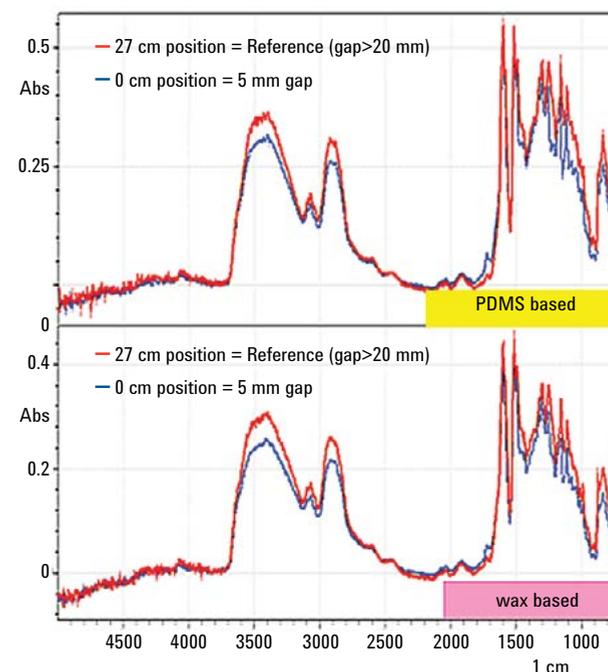
**Figure 4.** Infrared spectra of residual PDMS and wax release agent atop CFRP. The PDMS and wax formulations share some similarities spectrally since the PDMS formulation contains many wax-based compounds as well as PDMS.
