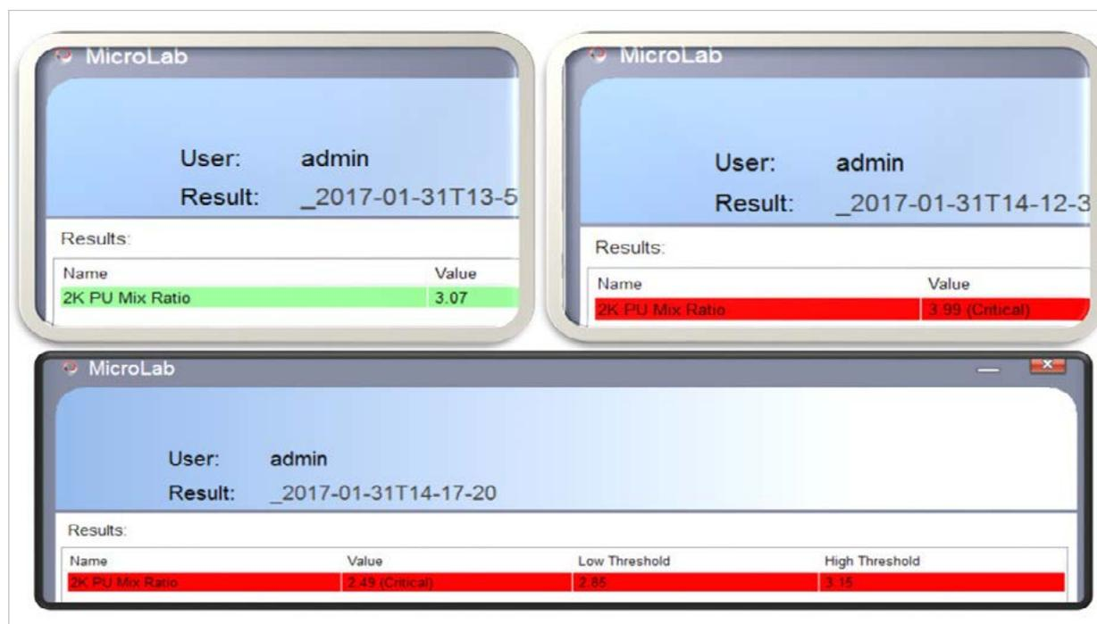
**Figure 5.** The visual display of the Agilent 4300 FTIR can display color-coded results, based on whether they are in or out of specification. Three example displays are shown here. (Top left). In-specification results are displayed in green. (Top right) Out of specification results highlighted in red (in this case, the resin rich sample). (Bottom) The specification limits can be adjusted in the method—this screens shows the upper and lower thresholds (flagging the resin poor sample).
