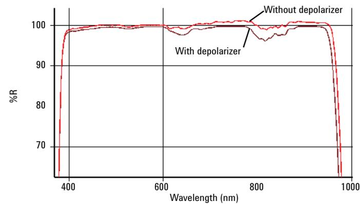
**Figure 6:** Demonstration of the importance of using a depolarizer after the sample but before the detector. Absolute reflection of backlight material at 30° s-polarized with a depolarizer before the detector (brown) and 30° s-polarized WITHOUT a depolarizer before the detector (red)
