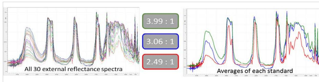
**Figure 3.** (Left) 3 x 10 external reflectance spectra of the three different ratios. (Right) The average of each 10 spectra, collected from the three coupons. The key to the color-coding of the spectra is shown to the left. Each individual spectra is the cumulation of 128 spectra ran at 4cm<sup>-1</sup> resolution taking only 40 s per spectra.
