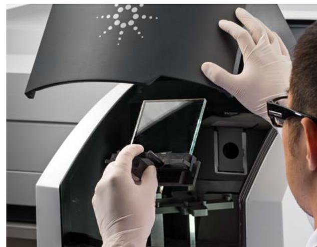
The revolutionary Agilent Cary 7000 Universal Measurement Spectrophotometer (UMS) can collect hundreds of UV-Vis-NIR spectra overnight, or characterize optical components or thin films in minutes to hours rather than hours to days.
