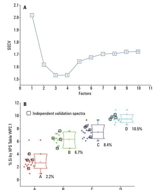
Figure 3. Standard error of cross validation versus number of factors (A), four treatment levels, and their partial least squares predicted values (B). The boxed black values are the validation spectra set aside to independently test the partial least squares model.
