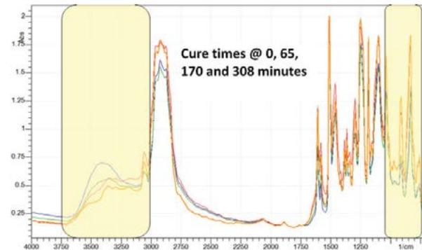
**Figure 2.** Room temperature cure of Epoxy/Hardener coating at 0 (orange), 65 (red), 170 (green) and 308 (blue) minutes. Highlighted areas show changes as the mixture cures and can be used to measure cure level directly once a correlation has been set up
