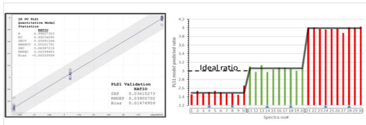
**Figure 4.** Left. Actual paint component ratios vs values calculated by the model. Right. The paint component ratio, calculated from 24 of the spectra collected. The asterisks (in both graphs) are the independent validation spectra that were not used to create the final model. The black dotted line indicates the ideal ratio of 3:1.
