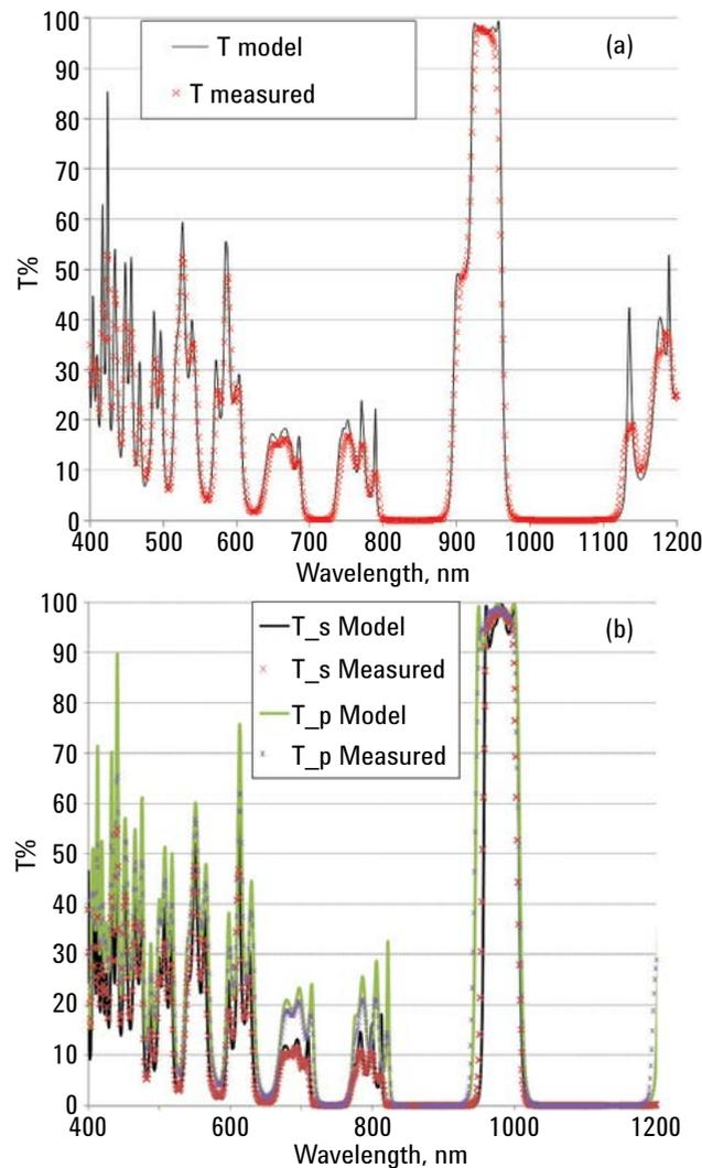
**Figure 2.** Comparison of oblique incidence experimental transmittance data for the sample BS-AR-Suprasil with model transmittance (a) non-polarized light at  $45^\circ$ , (b) s- and p-polarizations at  $30^\circ$
