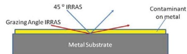
**Figure 1.** Diagram showing the sample interface of infrared reflection absorption spectroscopy (IRRAS) in both the grazing angle (red) and specular reflectance (blue) geometries. The grazing angle geometry has an increased pathlength through the contaminant
