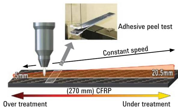
**Figure 2.** Plasma nozzle traverses CFRP coupon at fixed speed at continually decreasing distance from surface to induce temperature variation. Smallest plasma gap from surface creates highest temperature conditions. G1c value is collected from the adhesion peel measurements that were made with an Instron 5566 Universal Testing Machine. The CFRP laminate is 270 mm long. Two sections are bonded together with adhesive for the peel test.
