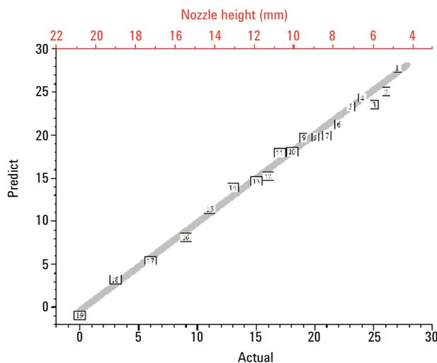
**Figure 5.** PLS multivariate analysis correlating infrared spectra as a function of position (i.e., nozzle height and temperature) on CFRP coupon for the PDMS based release agent. The cross-validated PLS model used three factors in the final optimized prediction model.
