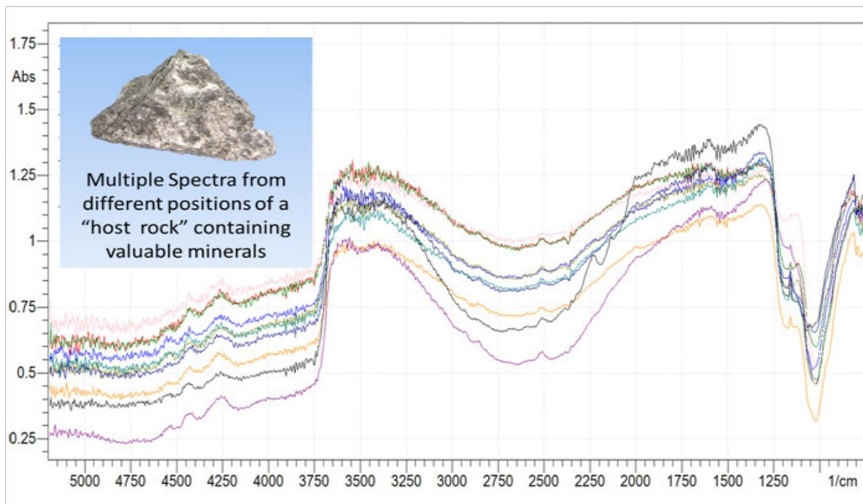
**Figure 3.** Diffuse reflectance spectra collected at 11 different locations on the surface of a geological monolithic ore rock fragment. Spectra were collected using an Agilent 4300 hand-held FTIR in conjunction with the diffuse reflectance interface option.
