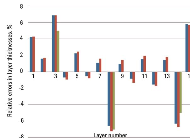
**Figure 2.** Comparison of errors in layer thicknesses of 15-layer quarter-wave mirror found on the basis of reflectance and transmittance data taken at 7°, 10°, 20°, 30°, and 40°, for the s-polarization case (blue bars) and the p-polarization case (red bars). Green bars show planned errors in the thicknesses of the third, eighth, 14th, and 15th layers.
