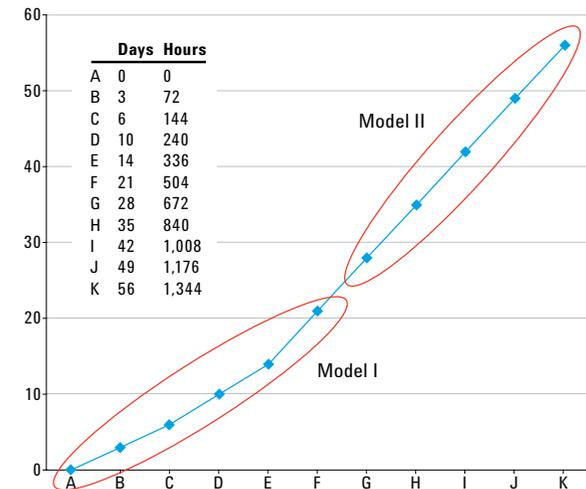
Figure 5. FTIR PLS Model I covers changes in the induction-to-middle exposure period. Model II covers the changes in the medium-to-end-of-life exposure period.
