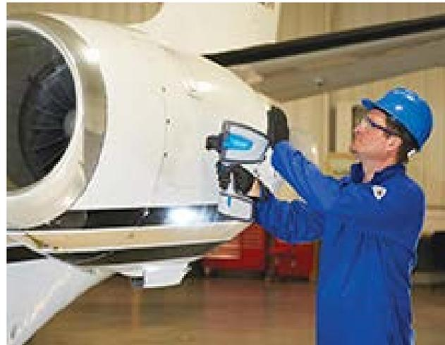
The handheld 4300 FTIR unit can be used insitu, anywhere, anytime. Instead of taking coating samples back to the lab, you can take non-destructive measurements of the coating on whatever it’s been applied to – walls, aircraft, glass etc.
