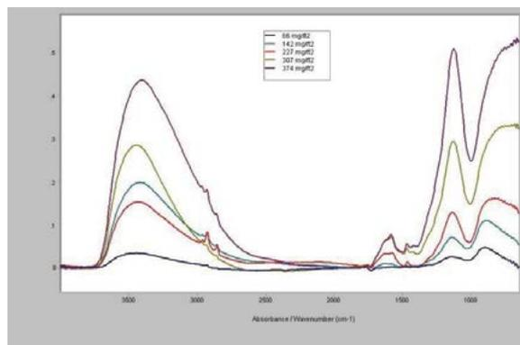
**Figure 1.** Spectral overlay of BSAA on 2024 aluminum calibration standards. Spectra were measured with 32 scans at 8 cm<sup>-1</sup> resolution with the Agilent 4100 ExoScan FTIR using external reflectance
