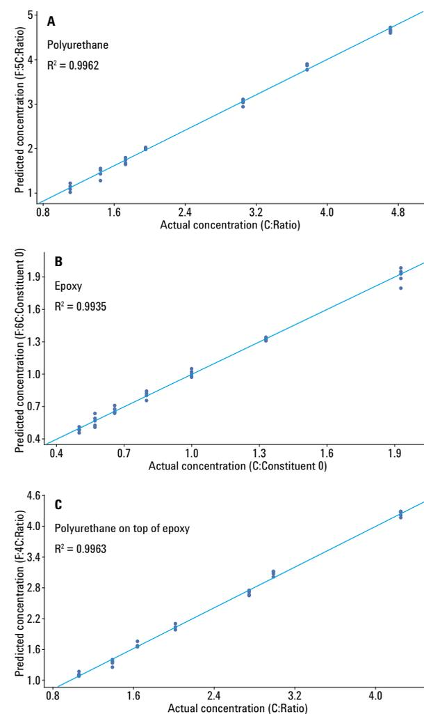
Figure 1. Calibration model obtained for different mix ratios of two-part coating systems (polyurethane, epoxy, and polyurethane on top of epoxy), developed using the PLS algorithm.
