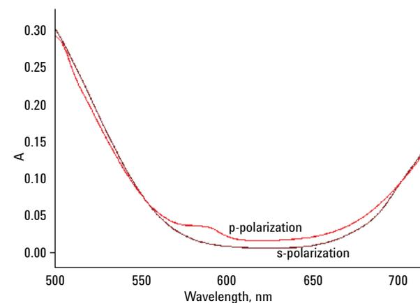
**Figure 6.** Absorbance spectra for s- and p-polarization
