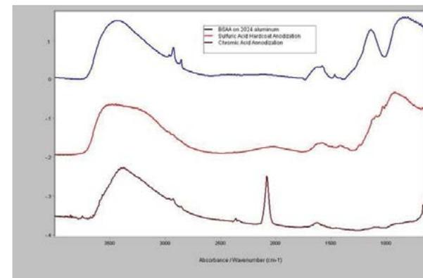
**Figure 5.** IR spectra of BSAA anodization (blue), sulfuric acid hardcoat (red) and chromic acid anodization (brown)
