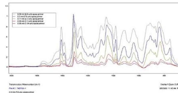
**Figure 2.** IR spectra collected with the Agilent 4100 ExoScan FTIR using the external reflectance sample interface of epoxy primer on aluminum sheet ranging in thickness from 0.06 mils (1.54 microns) to 0.39 mils (9.9 microns)
