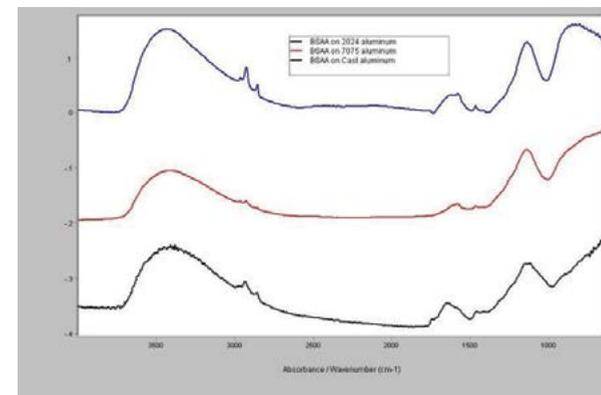
**Figure 4.** Comparison between spectra of BSAA on 2024 aluminum (blue), 7075 aluminum (red) and rough cast aluminum (black)
