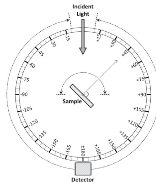
**Figure 1.** The AOI on the sample and the detector position can be set independently with 0.02° resolution. The AOI on the sample ranges from  $-85^\circ \leq \text{AOI} \leq 85^\circ$ . The detector can be placed at angles ranging from  $-10^\circ$  to  $10^\circ$ . As a result the Cary 7000 is able to determine R over the range  $5^\circ \leq |\text{AOI}| \leq 85^\circ$  and T over the range  $0^\circ \leq |\text{AOI}| \leq 85^\circ$ .
