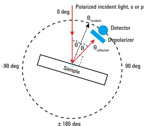
**Figure 3.** Schematic of the Cary 7000 UMS. Light incident onto the sample can be s, or p polarized. The detector module allows mounting of a depolarizer immediately before the detector. Absolute specular reflection of transmission can be measured
