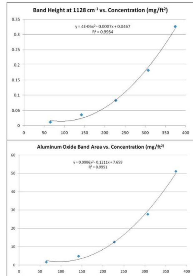
**Figure 2.** Calibration curves showing the aluminum oxide band height at 1128 cm<sup>-1</sup> versus concentration (top) and the aluminum oxide band area from 1390 cm<sup>-1</sup> to 995 cm<sup>-1</sup> versus concentration (bottom). Both calibration curves are fit by a quadratic equation with an excellent correlation coefficient.
