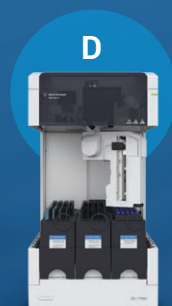
Agilent 1290 Infinity II Preparative Open-Bed 샘플러 / 분취기
