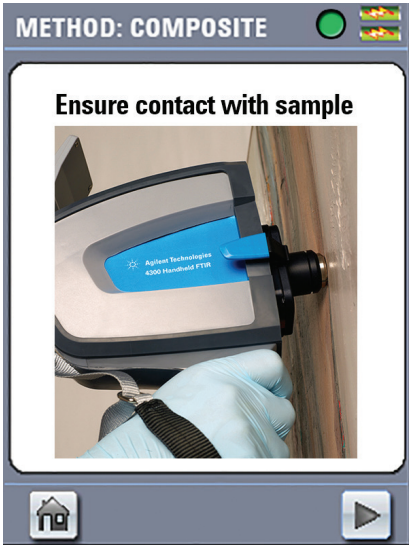
Agilent MicroLab software will instruct when to position the spectrometer's sample interface on the object to be analyzed.
