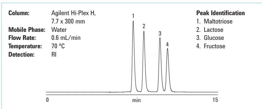
For carbohydrate analysis of samples containing high levels of organic acids, Agilent Hi-Plex H columns deliver sharp, reproducible peaks. Note, however, that some sugars (such as raffinose) can undergo acid hydrolysis even when water is used as the eluent.
