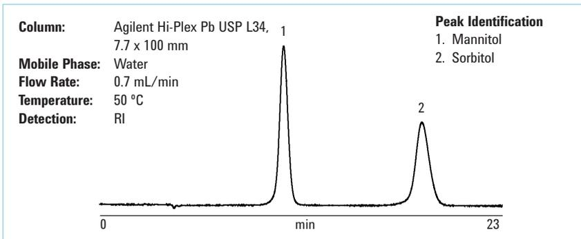
USP method for sorbitol – a sugar alcohol and alternative sweetener – using mannitol as the internal standard. Agilent Hi-Plex Pb columns are recommended for alcoholic drinks that also contain glycerol, as well as sweetened dairy-based food products.
