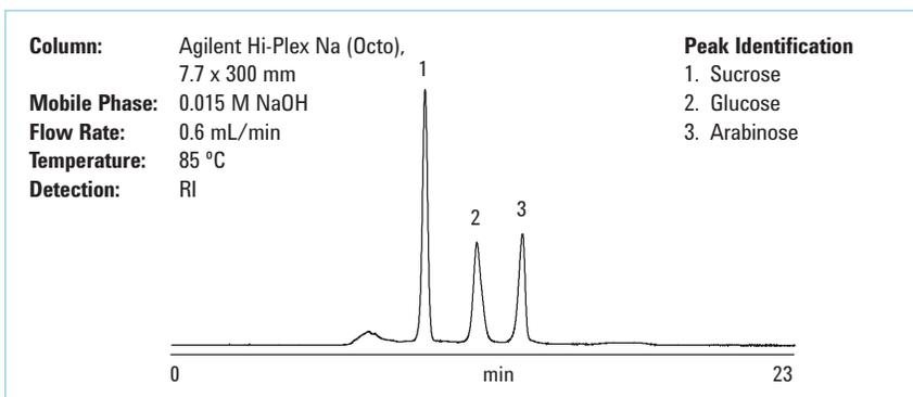
Food products containing high levels of sodium ions are best analyzed with Agilent Hi-Plex Na (Octo) columns. This saves time when sodium hydroxide is used as the eluent with PAD, because it eliminates the need for the post-column addition of sodium hydroxide.
