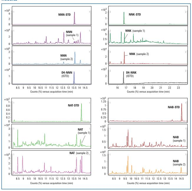
MRM chromatograms of TSNA standard solution and the real samples using an Agilent 7000A Triple Quadrupole GC/MS system and an Agilent J&W DB-35ms Ultra Inert  $0.25 \text{ mm} \times 30 \text{ m}$ ,  $0.25 \text{ }\mu\text{m}$  column.
