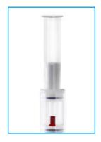
Solid supported extraction on Agilent Chem Elut cartridges.
