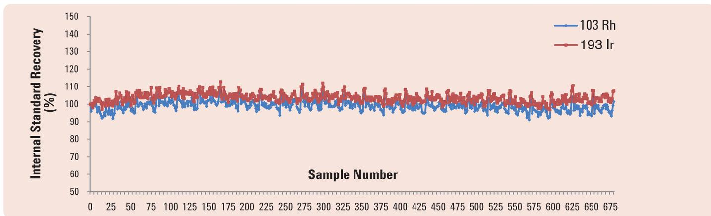
Figure 2. Internal standard recovery for the entire sequence of ~700 high-matrix rock digests, showing excellent stability throughout the sequence
