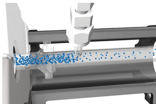
Figure 1. Schematic of HMI, showing aerosol dilution
