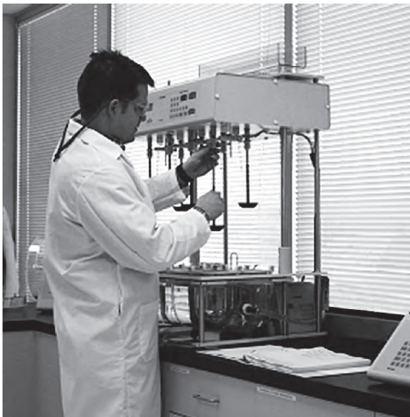
Figure 6. Typical dissolution setup.
