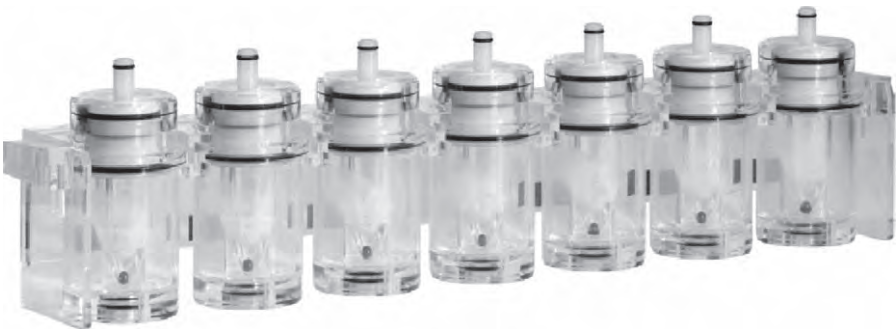
Figure 20. Set of USP Apparatus 4 flow-through cells.
