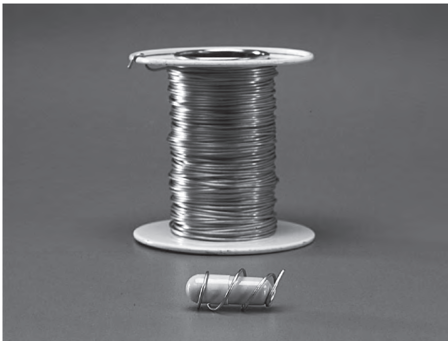
Figure 9. Sinker constructed of stainless steel wire.
