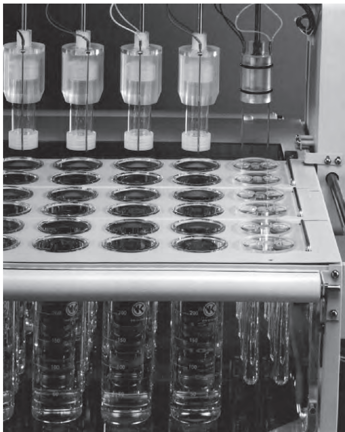
Figure 18. Typical Bio-Dis setup.
