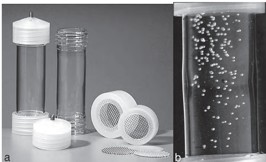
Figure 17. Bio-Dis reciprocating cylinder inner tubes.
