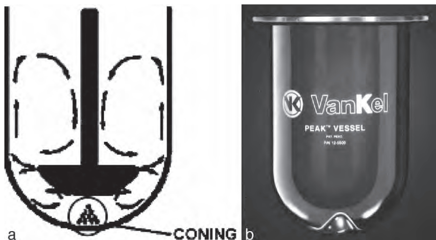
Figure 12. Cone formation (12a) and Peak vessel configuration (12b).
