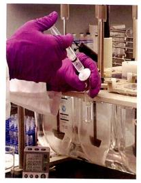
Figure 2. Filtration of the dissolution sample.
