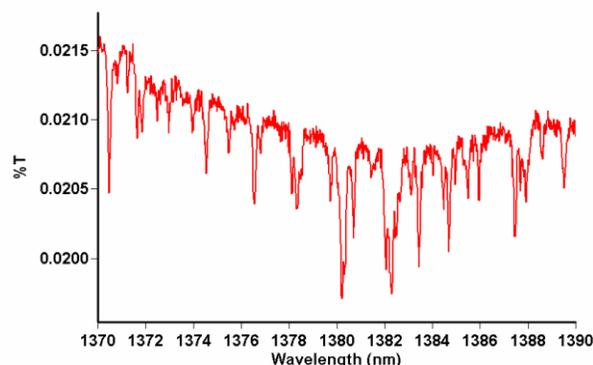
Figure 1. Water vapor transmission spectrum collected on a Cary 5000 spectrophotometer
