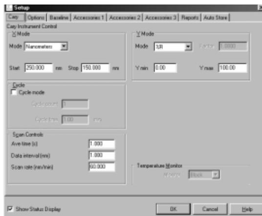
Figure 3. Instrumental parameters for optical coating measurement
