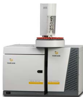
Figure 2. Varian 220-MS ion trap mass spectrometer with 431-GC gas chromatograph and CP-8400 AutoSampler.
