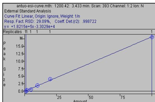
Figure 7. Calibration curve for ANTU from 1 to 125 ppb. The  $r^2$  value is 0.998.
