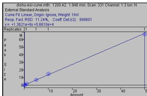
Figure 6. Calibration curve for diphacinone from 0.2 to 50 ppb. The  $r^2$  value is 0.999.
