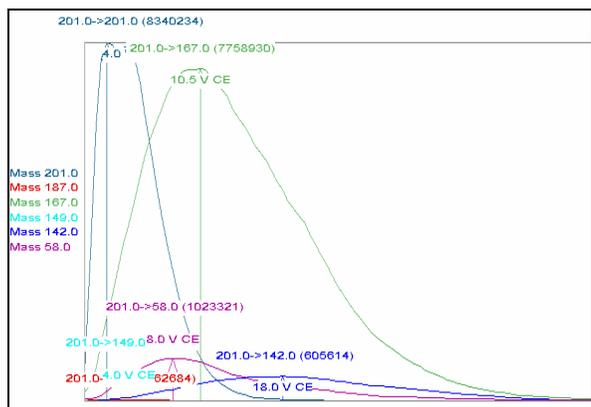
Figure 2. MS/MS breakdown curve for ANTU.
