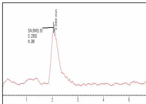
Figure 5. Chromatogram of diphacinone at 0.2 ppb. The S/N ratio is 83.
