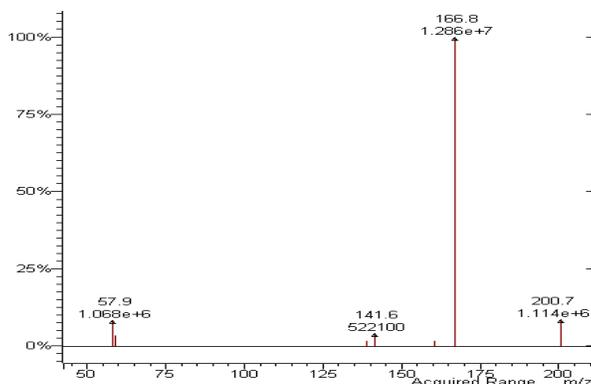
Figure 3. The MS/MS product ion spectrum for ANTU. The parent ion is  $m/z$  201, and the most abundant product ion is  $m/z$  167.
