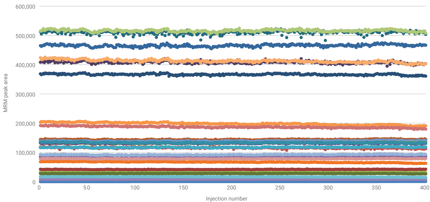
Figure 3-9. Method robustness for 25 representative vet drugs responses over 400 injections of milk samples prepared by Agilent Captiva EMR-Lipid passthrough cleanup after solvent extraction.
