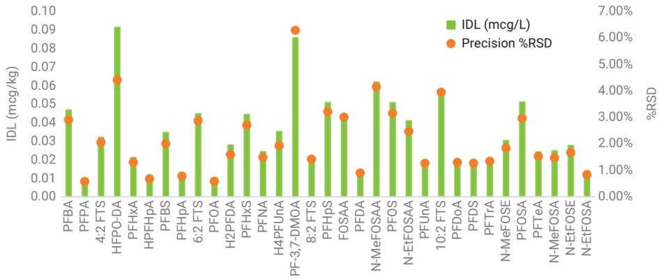
Figure 5. Instrument detection limits (IDLs).
