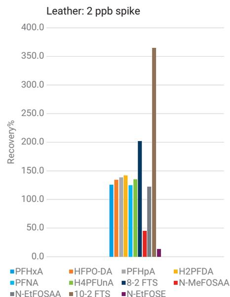
Figure 8. Recovery for the PFAS spiked at 2 µg/L into a leather extract. The PFAS were quantified using external solvent calibration curves.
