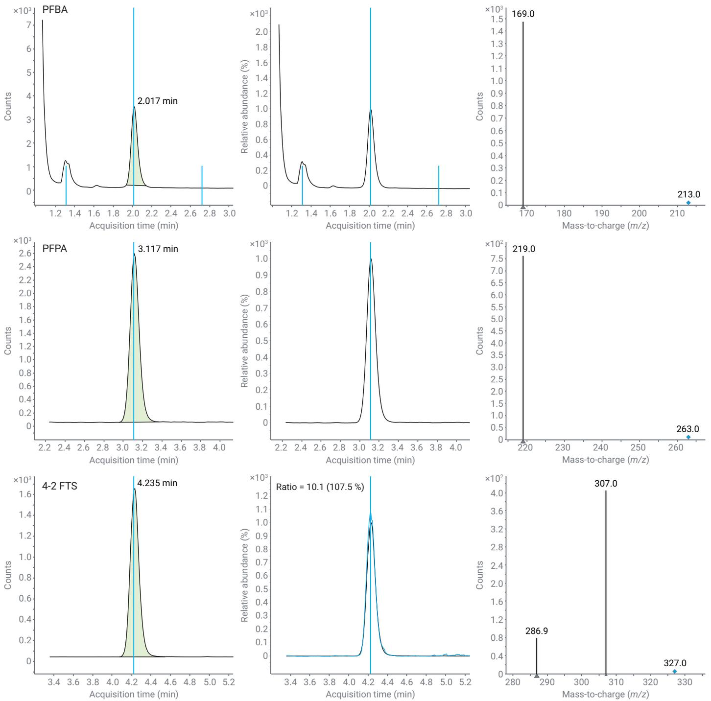
**Figure 4.** Chromatograms of PFAS (PFBA, PFPA, and 4:2 FTS) at 1 µg/L used for IDL calculations.
