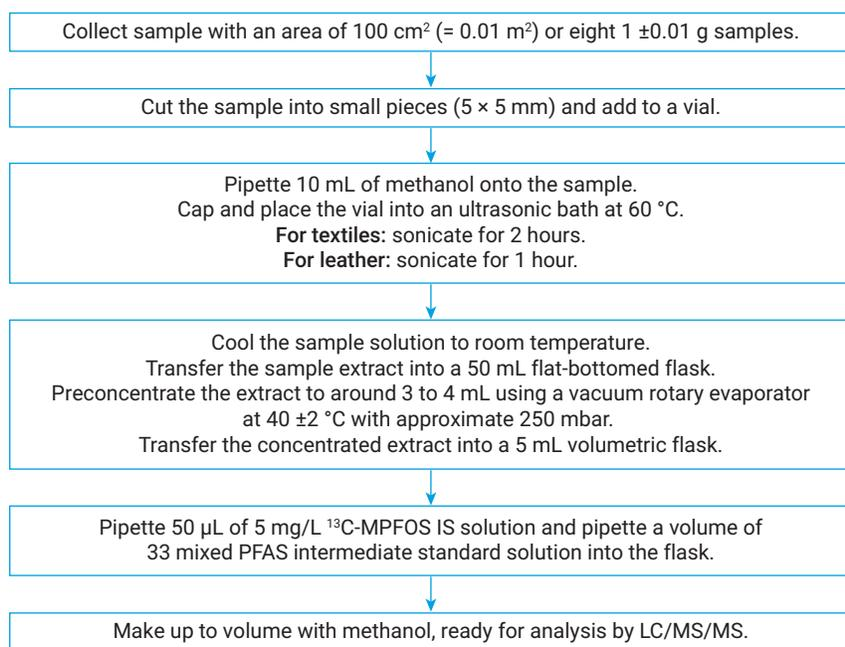
**Figure 1.** Sample preparation procedure for the extraction of PFAS from textiles and leather.
