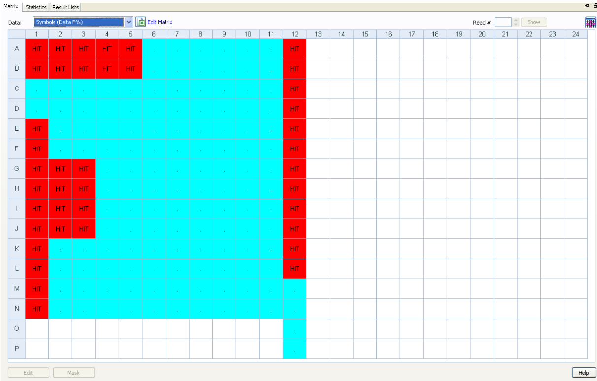
Figure 3. Results from Cutoff Analysis of inhibition data. Wells showing Delta F(%) values \leq 50\% of maximum stimulated wells labeled in red. All other wells labeled in green.
