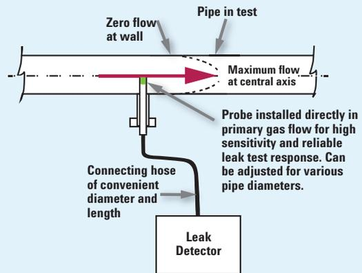
Figure 2: Gas flow characteristics and the effect on sampling
