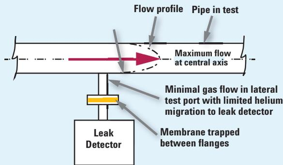
**D – using an insertable membrane probe to sample in the center of the pipe**
