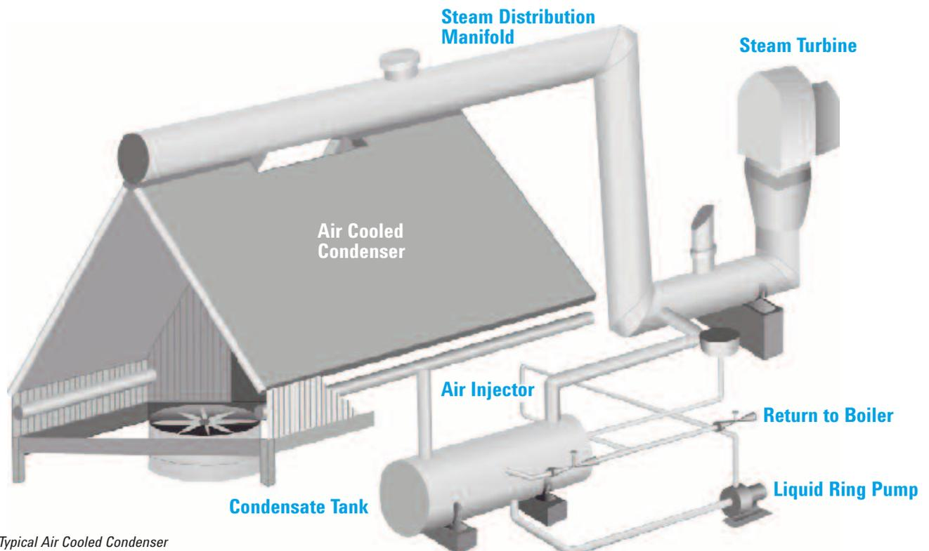
Figure 1: Typical Air Cooled Condenser
