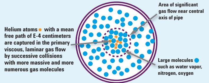
**C – sampling with a membrane mounted on the side wall of the pipe**
