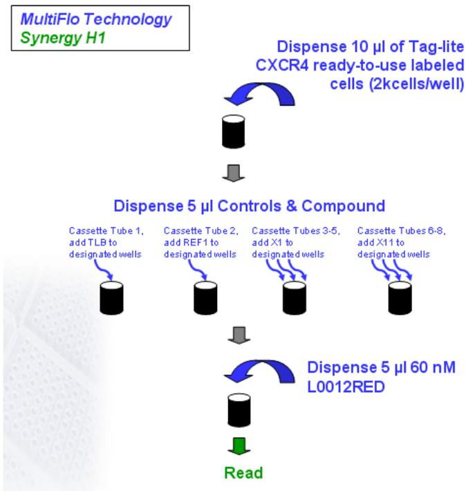
Figure 4. HTS simulation workflow.
