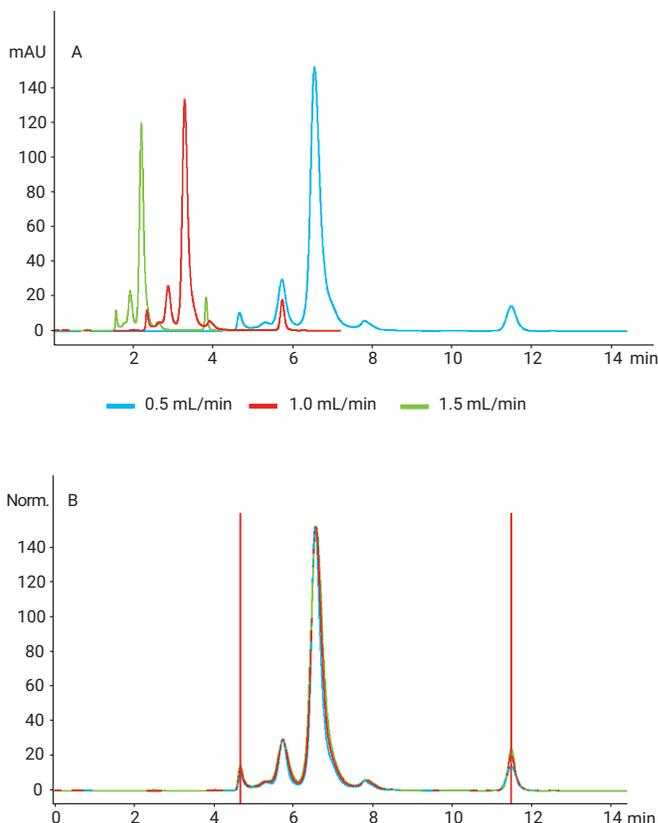
**Figure 10:** Increasing the flow rate reduces the analysis time from 12 to 4 minutes (A). When the retention times are normalized and overlaid (B) it is evident that the retention times are consistent and that there is minimal reduction in resolution.
