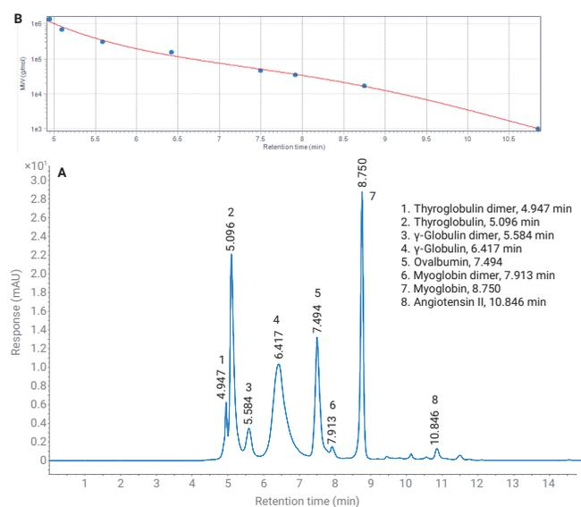
**Figure 1.** (A) Separation of a five-protein mixture including three dimers on the Agilent AdvanceBio SEC, 200 Å, 4.6 × 300 mm, 1.9  $\mu\text{m}$  in combination with the Agilent 1290 Infinity II Bio Ultra Low Dispersion Kit comprising 0.07 mm capillaries. (B) Calibration curve of SEC for molecular weight determination with a protein mixture featuring some dimers.
