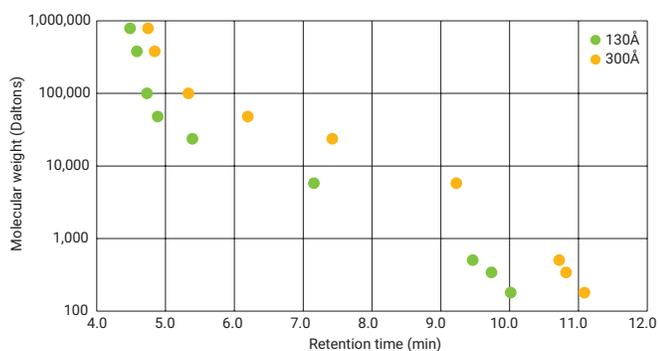
**Figure 4.** Polysaccharide calibration on Agilent AdvanceBio SEC columns.
