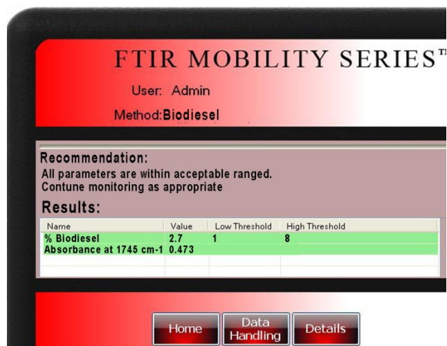
Figure 4. MicroLab results screen for a 3.0% sample of biodiesel in diesel
