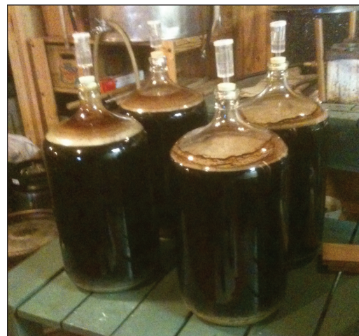
Figure 1. Glass fermentation carboys. Small batch brewing methods often employ the use of glass containers with liquid air-lock systems.
