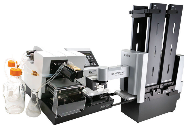
Figure 6. Agilent BioTek EL406 semi-automated systems. Agilent BioTek EL406 washer dispenser integrated with an Agilent BioTek BioStack 4 robotic device.
