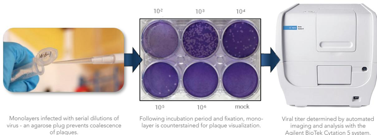
**Figure 1.** Viral plaque assay workflow incorporating automated imaging and analysis conducted with the Agilent BioTek Cytation 5 cell imaging multimode reader and Agilent BioTek Gen5 microplate reader and imager software.
