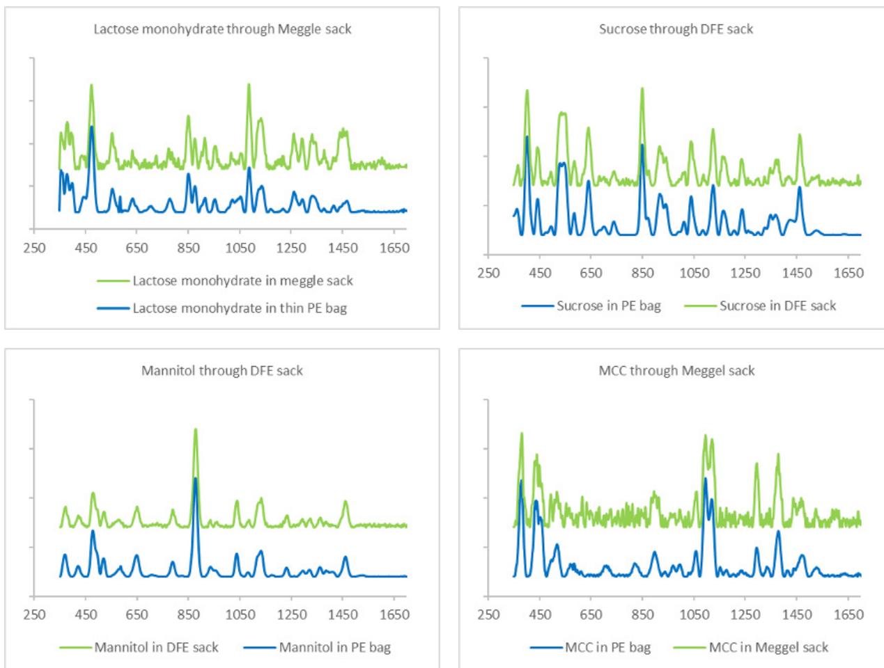
Figure 2. Sucrose and mannitol through a DFE sack, MCC and lactose monohydrate through a Meggle sack. SORS spectra overlaid with sucrose, mannitol, MCC, and lactose monohydrate Raman spectra through a polyethylene liner.
