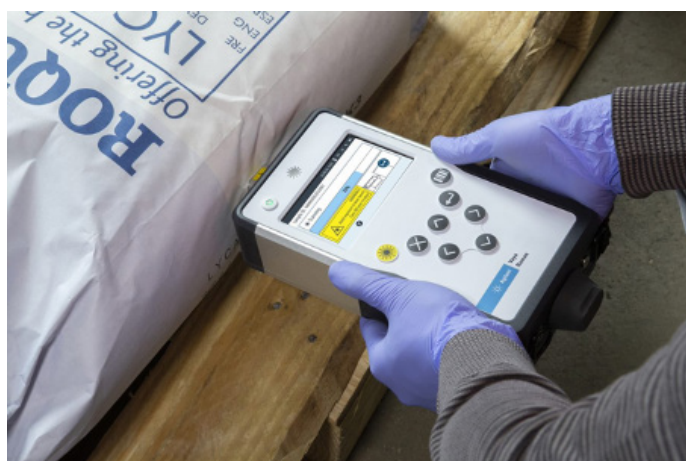
Figure 1. Using a Vaya Raman instrument to identify contents through a multilayer paper sack.
