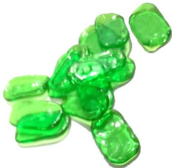
**Figure 1.** Empty soft gel capsules used to prepare the calibration standards.
