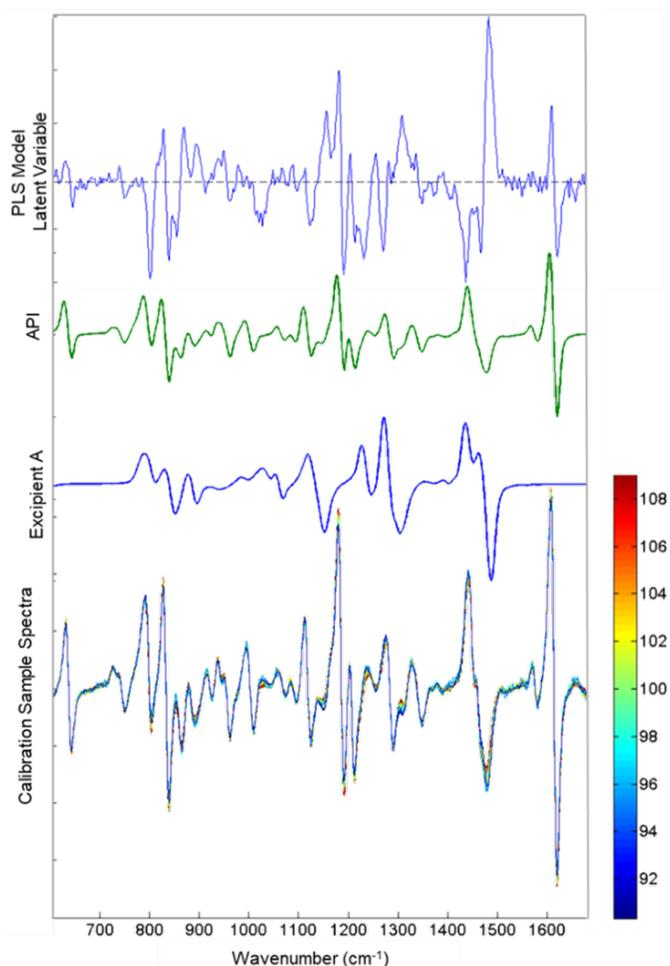
Figure 4. From bottom to top: calibration spectra colored according to API concentration 1<sup>st</sup> derivative SNV, excipient A, API 1<sup>st</sup> derivative SNV, and PLS model latent variable 1.
