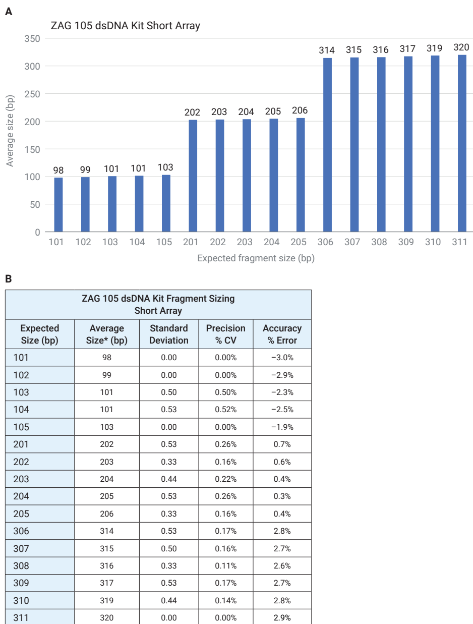
Figure 1. DNA fragments analyzed on the Agilent ZAG DNA Analyzer system with the short array and the Agilent ZAG 105 dsDNA kit (1-500 bp). (A) Average size of each single fragment. (B) Excellent precision and accuracy of the single fragments. *n = 9.
