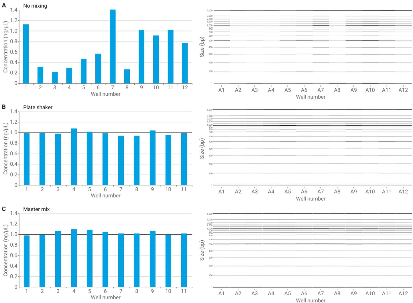
**Figure 1.** A complete row of Agilent HS NGS DNA Ladder was run on the Agilent 5200 Fragment Analyzer system with the Agilent HS NGS Fragment kit (1-6000 bp). Bar graph and gel image. (A) No mixing of the ladder and diluent marker in the plate. (B) Mixing by plate shaker. (C) Master mix of ladder and diluent marker vortexed in a low-bind tube and then pipetted into each well. Mixing is required for reliable quantification of a sample. The known concentration was 1.025 ng/μL.
