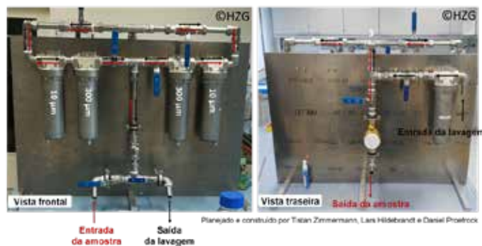
Figura 2. Frente e verso do Geesthacht Inert Microplastic Fractionator (GIMPF).
