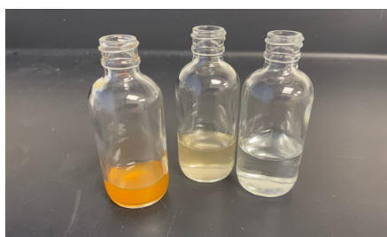
Figure 1. The lithium content of brine samples of varying concentrations was determined. Shown here are the undiluted samples.
