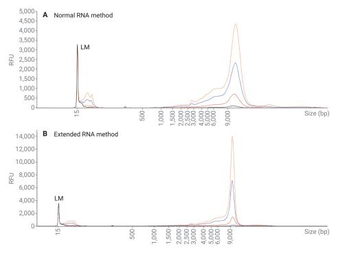
**Figure 3.** Overlay of the 10,000 nt IVT mRNA fragments over a dilution series of 100, 50, 10, 1 ng/ $\mu$ L separated on the Agilent 5200 Fragment Analyzer system with the Agilent RNA kit (15 nt) using the long RNA Ladder and (A) the normal RNA method (B) the extended RNA method. LM = lower marker.
