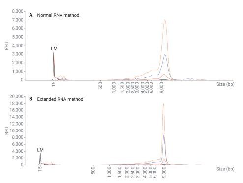
**Figure 2.** Overlay of the 9,000 nt IVT mRNA fragments over a dilution series of 100, 50, 10, 1 ng/ $\mu$ L separated on the Agilent 5200 Fragment Analyzer system with the Agilent RNA kit (15 nt) using the long RNA Ladder and (A) the normal RNA method (B) the extended RNA method. LM = lower marker.
