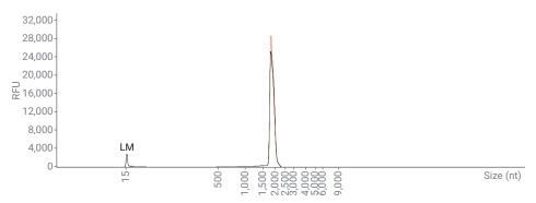
**Figure 5.** Overlay of the 1,800 nt IVT mRNA fragments capped (red) and uncapped (black) separated on the Agilent 5200 Fragment Analyzer system with the Agilent RNA kit (15 nt) using the extended RNA method and the long RNA Ladder. LM= lower marker
