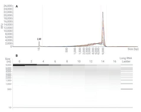
**Figure 4.** 9,000 nt IVT mRNA analyzed on the Agilent 5200 Fragment Analyzer system with the Agilent RNA kit (15 nt) using the long RNA Ladder and extended RNA method over a degradation series at 70 °C from 0 to 16 minutes. (A) Electropherogram overlay of degradation series. (B) Gel image of degradation. LM = lower marker.
