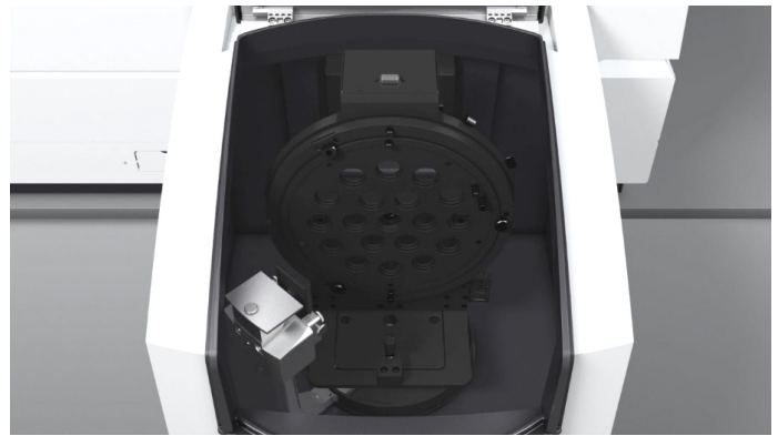
Figure 1a. Plan view of the Cary 7000 UMS measurement chamber with the Solids Autosampler installed.
