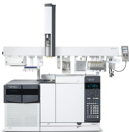
Figure 2. The PAL RTC rail system combined with an Agilent 7890B GC and an Agilent 5977B GC/MSD.
