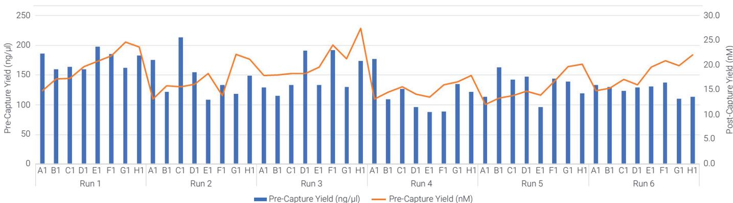
**Figure 2.** Comparison of pre and post capture yield obtained during six validation runs on the MagnisDx system. 50 ng of mechanically sheared FFPE DNA was used as input. PCR cycle numbers for pre- and post-capture amplification were 13 and 9 cycles, respectively. Pre-capture yield for each sample is shown in the blue bars, while post-capture yield is shown as an orange line. Overall, there is good consistency between samples across the runs.
