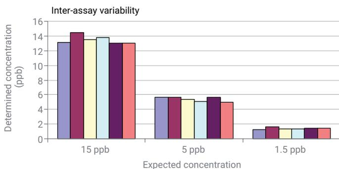
**Figure 4.** Inter-assay repeatability. Multiple replicates of samples at three different concentrations were assayed individually on the same microplate. The absorbance values for each sample were then used to interpolate a standard curve. The resultant calculated concentrations were exported to Microsoft Excel via the Power Export function of Agilent BioTek Gen5 and plotted.
