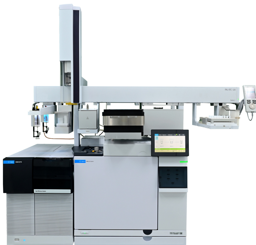
Figure 1. PAL3 Series 2 RTC autosampler with Agilent 7010D triple quadrupole GC/MS.
