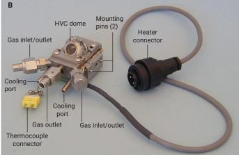
Figure 2. (A) Praying Mantis diffuse reflectance accessory. (B) High temperature reaction chamber for the Praying Mantis.
