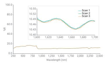
**Figure 4.** Three repeated wavelength scans of PTFE powder acquired at RT using the Agilent Cary 5000 UV-Vis-NIR spectrophotometer. The inset shows the wavelength region between 1,600 and 1,700 nm, highlighting the repeatability of the measurements.
