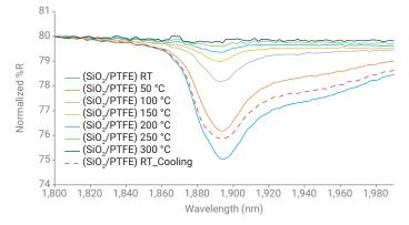
**Figure 5.** Diffuse reflectance spectra of  $SiO_2$  measured at different temperature points from RT to 300 °C. The dotted line represents the trace collected when the sample was allowed to cool down to room temperature.
