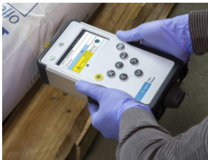
Figure 2. The Agilent Vaya Raman handheld spectrometer being used to identify materials inside paper sacks that typically comprise three layers of paper and a PE liner.
