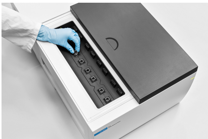
Figure 1. The Agilent Cary 3500 Multicell UV-Vis spectrophotometer has eight stationary cell positions and a double beam optical design with fiber optic technology and eight respective detectors, allowing simultaneous measurement of up to seven samples and a reference.
