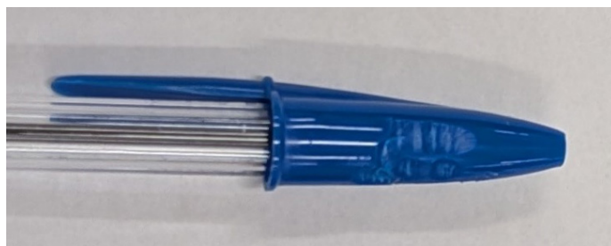
Figure 9. Pen cap tested with fast and conventional methods. Samples were sliced off from the middle of the cap as visible in the photo.
