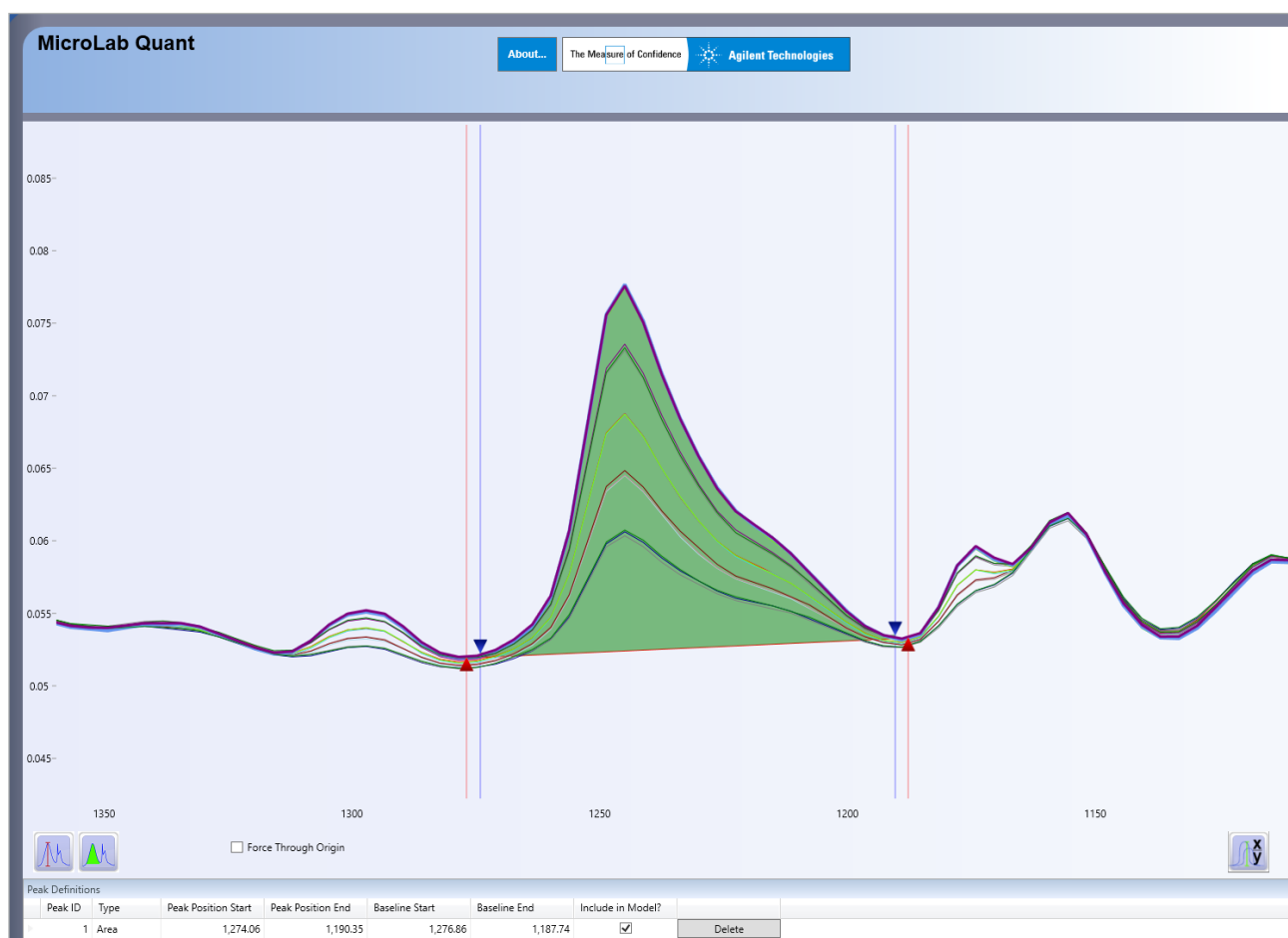
Figure 3. The Agilent MicroLab Quant application allows identifying the most suitable band for analyte quantification, enabling the optimization of analysis parameters such as peak position, and peak start and end points. The band at 1250 \text{cm}^{-1} for phenoxyethanol is distinct, making it suitable for calibration curve generation.
