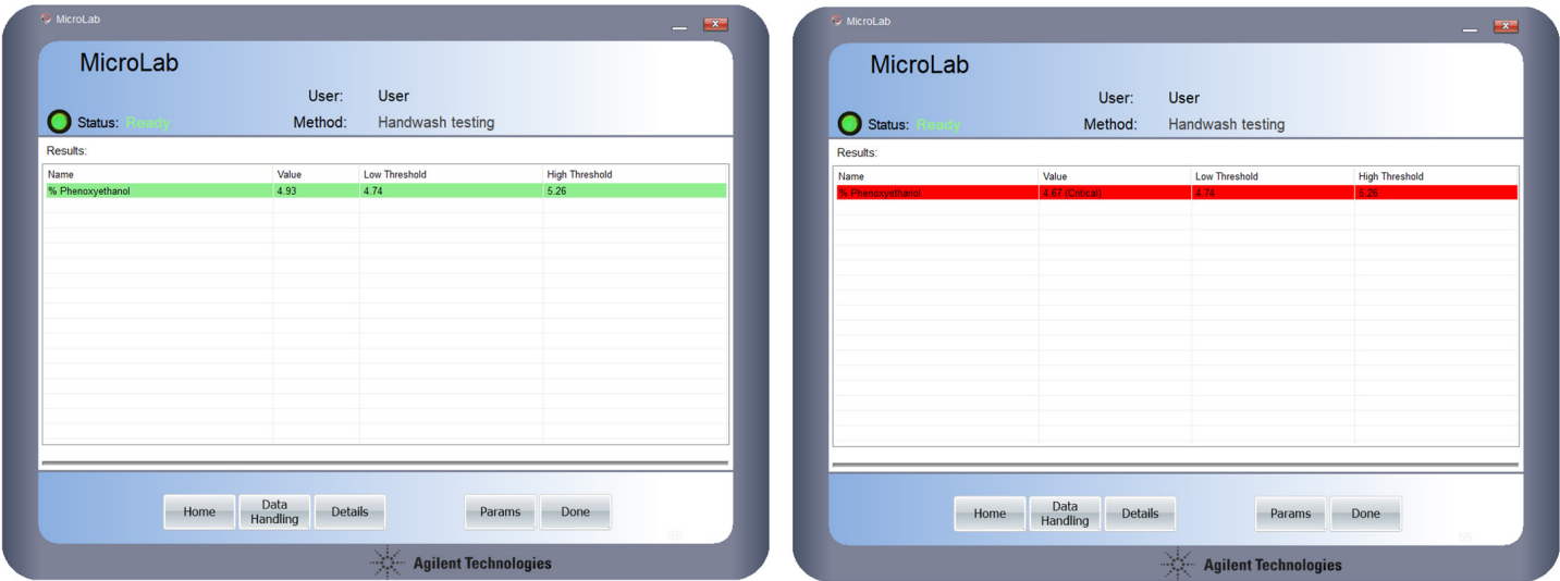
Figure 6. The integration of the Agilent Cary 630 FTIR-ATR quantification model into the Agilent MicroLab software method simplifies routine analysis of biocidal handwash batches. The software determines percentage concentration and provides color-coded, actionable results after data acquisition, highlighting in-spec samples in green and out-of-spec samples in red.
