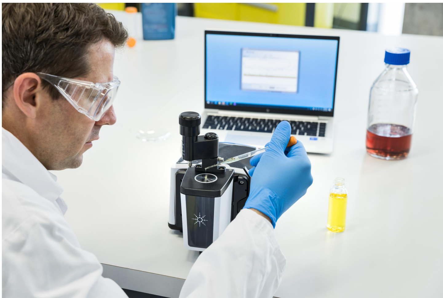
Figure 1. The Agilent Cary 630 FTIR spectrometer with diamond ATR module is ideal for the fast and easy quantification of phenoxyethanol in handwash products.
