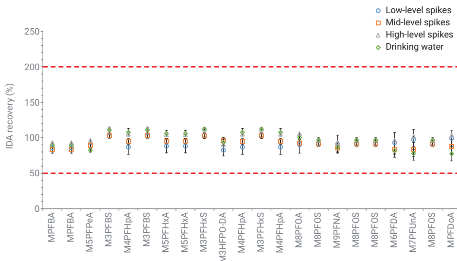
Figure 10. Absolute recoveries of IDAs in the low-level spikes, mid-level spikes, high-level spike, and drinking water samples.
