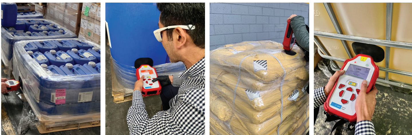
Figure 4. Operators analyze different consignments of agrochemicals using the Agilent Resolve handheld Raman analyzer.
