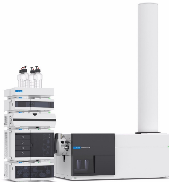
Figure 1. Agilent 6545XT AdvanceBio LC/Q-TOF and Agilent 1290 Infinity II Bio LC system.
