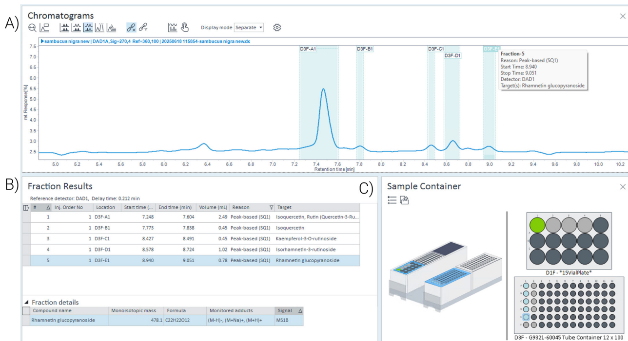
Figure 1. Fraction layout in OpenLab CDS data analysis. A) Chromatograms are highlighted with fraction collection regions. B) The fraction results table presents a tabular summary of the collected fractions and the triggering targets. C) The sample containers component highlights the sample vial used and the location of the collected fractions.
